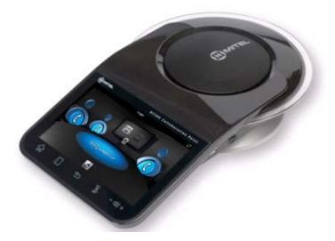
It has a patented beam forming microphone array that delivers 360° audio clarity to all participants. It automatically locates the talker in the room and attenuates background noise by adjusting the microphone sensitivity towards the current talker. It provides visual indication of the active speaker.
